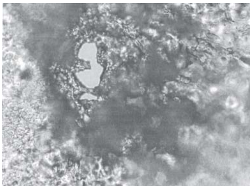
Fig. 6. Biodegradation of PVA/BC composite film after 176 days inside compost pot C recorded with camera-linked light microscope (20× magnification)
